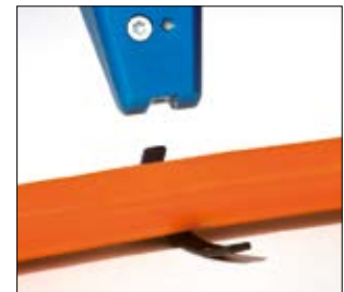
... release the button and remove the tool, the tie is cut.
