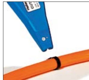
Bring the tool perpendicular to the tie...
