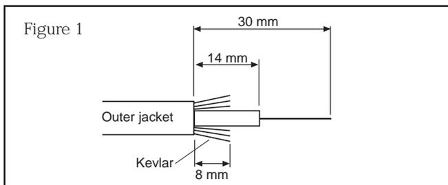
6. Using 2.5 or 3mm sheath dia. 125 micron fibre cable, slide the strain relief boot on, then the appropriate colour crimp ring (largest diameter facing towards the connector). Red ring for 2.5mm cable, black ring for 3mm cable. Strip and prepare as in Figure 1.
