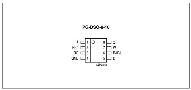
Figure 1 Pin Configuration (top view)
