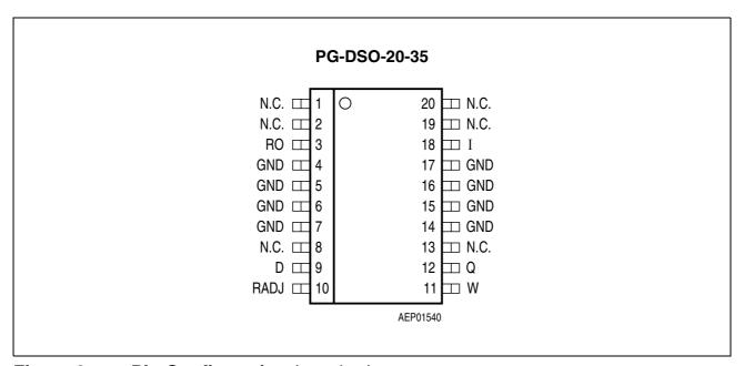
Figure 2 Pin Configuration (top view)
