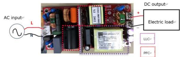
Figure 7. Wiring diagram of EVK
