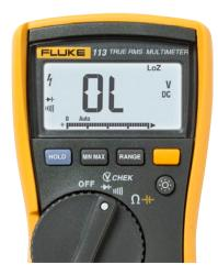
The Fluke 113 is now ready to make either a continuity test, diode check, or voltage measurement. All three tests are automatic. The meter will determine the correct measurement.
