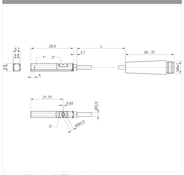
$1^*$  = switching point  $2^*$  = locking screw  $3^*$  = LED window, transparent
