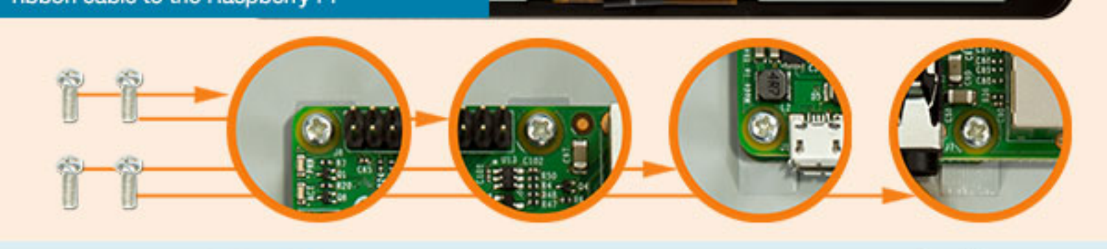
Use the 4 x screws to secure the Raspberry Pi board to the Standoffs then connect the DSI ribbon cable to the Raspberry Pi
