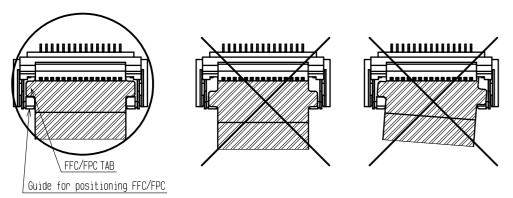
♦ Checking the Locking Condition
