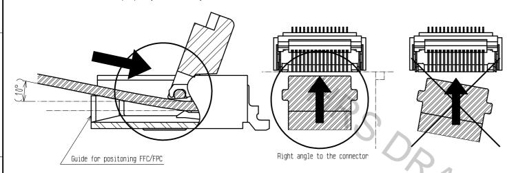
2. Do not insert the FFC/FPC diagonally from above.
