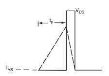
Fig. 12b - Unclamped Inductive Waveforms
