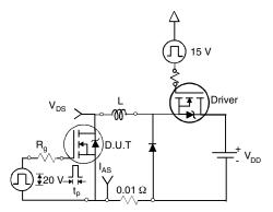
Fig. 12a - Unclamped Inductive Test Circuit
