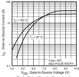
Fig. 3 - Typical Transfer Characteristics
