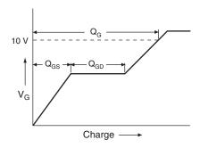
Fig. 13a - Basic Gate Charge Waveform
