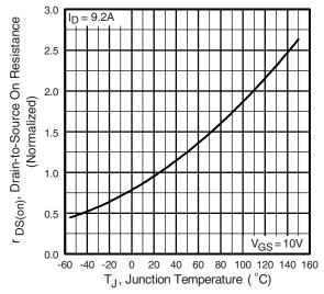
Fig. 4 - Normalized On-Resistance vs. Temperature
