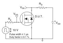
Fig. 10a - Switching Time Test Circuit
