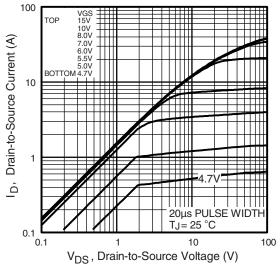
Fig. 1 - Typical Output Characteristics
