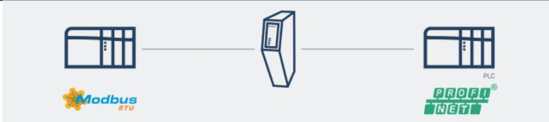
The Anybus Communicator Modbus RTU Server to PROFINET IO-device enables you to connect any Modbus RTU control system to any PROFINET control system.
