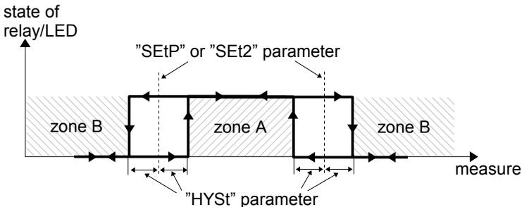
Figure 6.5. Two threshold control of the relay/LED outputs
