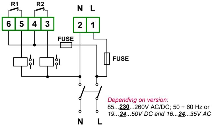
Figure 4.15. Connection of power supply and relays
