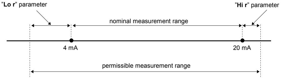
Figure 6.1. Definitions of measurement ranges in mode 4 ÷ 20mA
