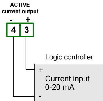
Figure 4.18. Example of active current outputs connection
