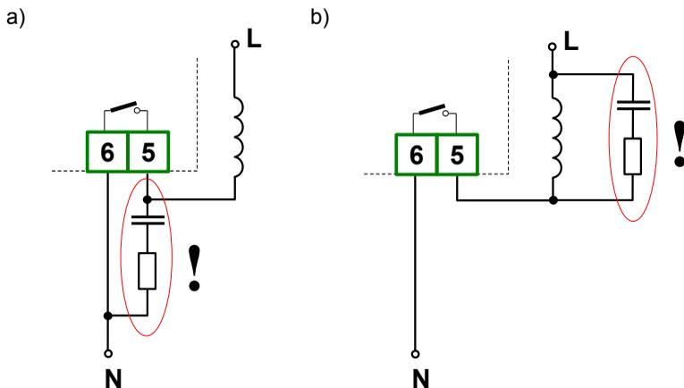
Figure 4.16. Examples of suppression circuit connection:
