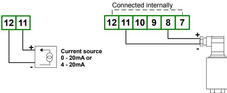
Figure 4.21. Connections of 2-wire sensor:
