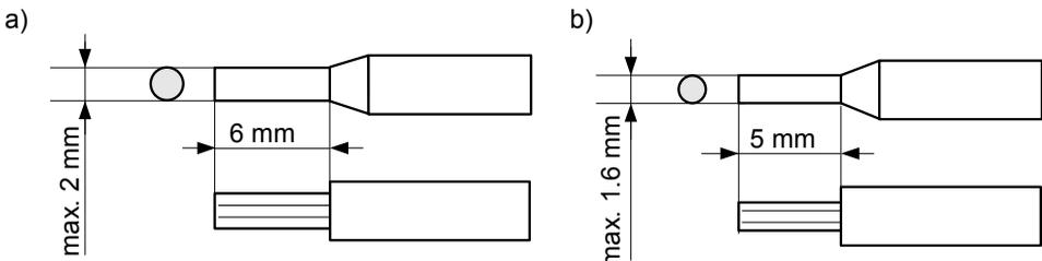
**Figure 4.2. Recommended dimensions of cable stripping**
