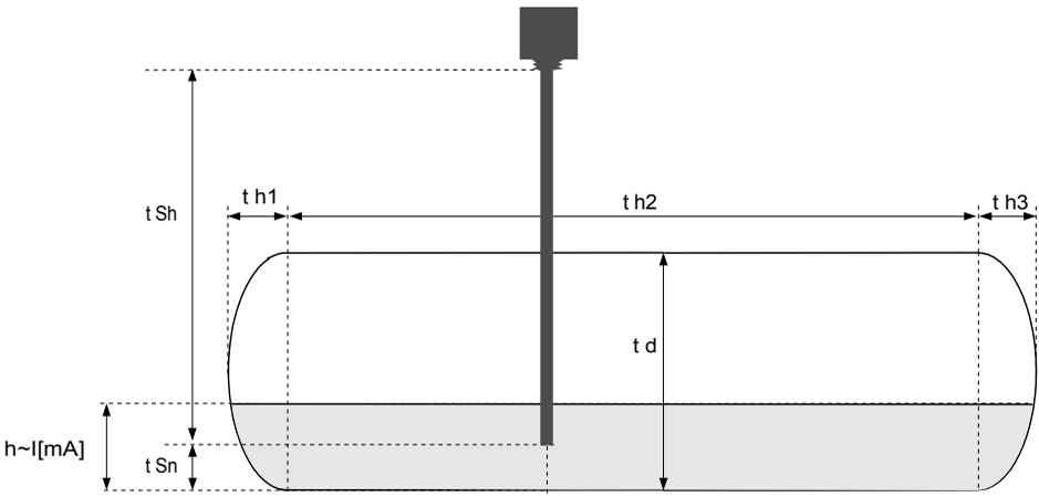
Figure 7.2 Parameters of cylindrical tank in horizontal position.
