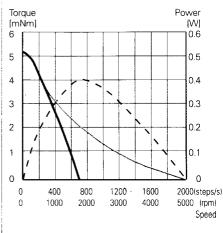
**P110-064-015,** U = 12V,  $Rs = 15\Omega$ **P110-064-068,** U = 24V,  $Rs = 68\Omega$ Voltage drive type L/R
