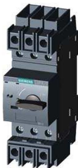
CIRCUIT-BREAKER SZ S00, FOR PLANT PROTECTION, WITH APPROBATION CIRCUIT-BREAKER UL 489. CSA C22.2 NO.5-02. A-RELEASE 15 A, N-RELEASE 208 A, SCREW CONNECTION, STANDARD SW. CAPACITY
