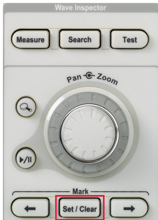
Figure 2B. Dedicated front-panel controls for setting/clearing marks and navigating between them.
