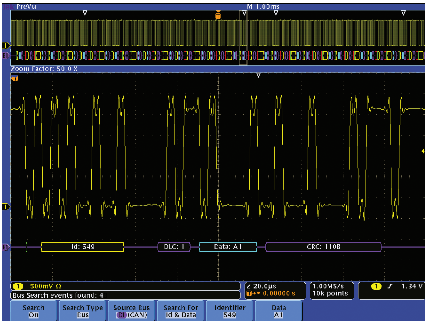
Figure 6. Searching for specific Identifier and Data values in CAN messages.
