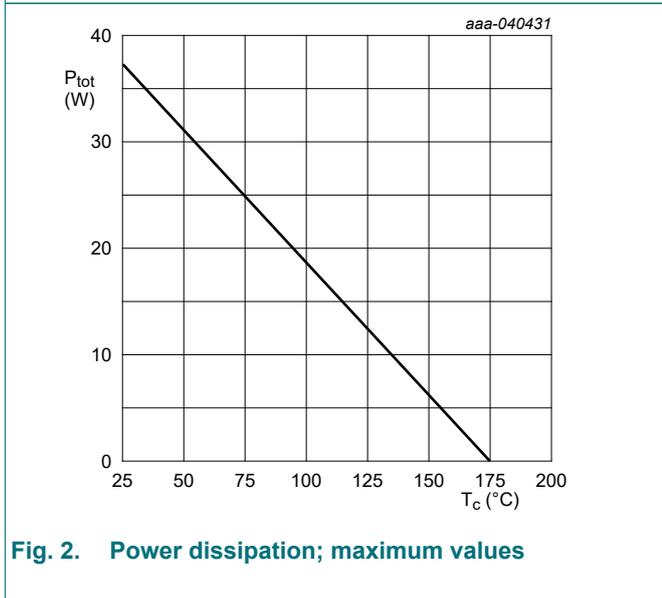
Fig. 2. Power dissipation; maximum values
