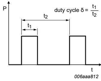
Fig. 10. Duty cycle definition
