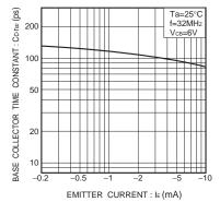
Fig.11 Base-collector time constant vs. emitter current
