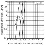
Fig.1 Grounded emitter propagation characteristics
