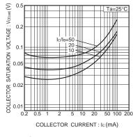
Fig. 6 Collector-emitter saturation voltage vs. collector current
