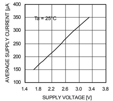
Fig.11 I<sub>DD</sub> – Supply voltage
