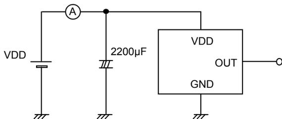
Fig.5 I<sub>DD</sub> measurement circuit
