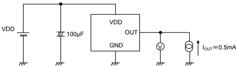
Fig.4 V<sub>OL</sub> measurement circuit
