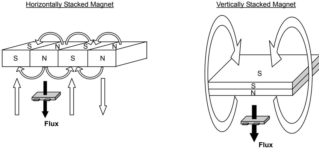
Because the field loop in horizontally stacked magnets extends for a shorter distance than that of vertically stacked magnets, the gap between the magnet and the hall IC must be decreased. Therefore, if horizontally-stacked magnets are used in the application, the thickness of the magnet or the area of each section should be increased to allow for a larger gap between the magnet and IC.
