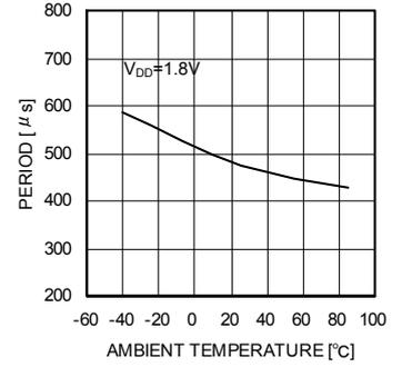
Fig.8 T<sub>P</sub>– Ambient temperature
