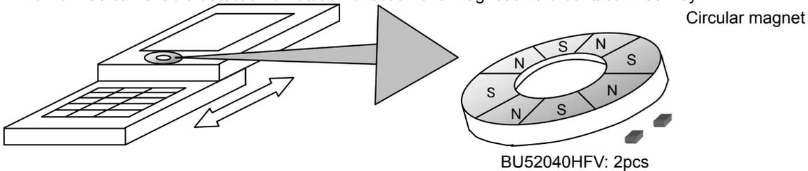
Mounting Position of Hall IC Inside Wheel Key
