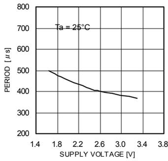
Fig.9 T<sub>P</sub>– Supply voltage
