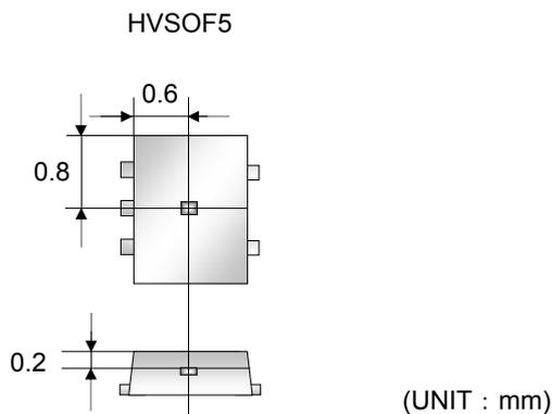
●Footprint dimensions (Optimize footprint dimensions to the board design and soldering condition)
