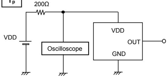
The period is monitored by Oscilloscope.
