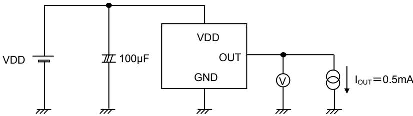
Fig.3 V<sub>OH</sub> measurement circuit
