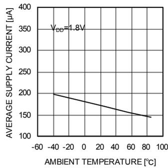
Fig.10 I<sub>DD</sub>– Ambient temperature
