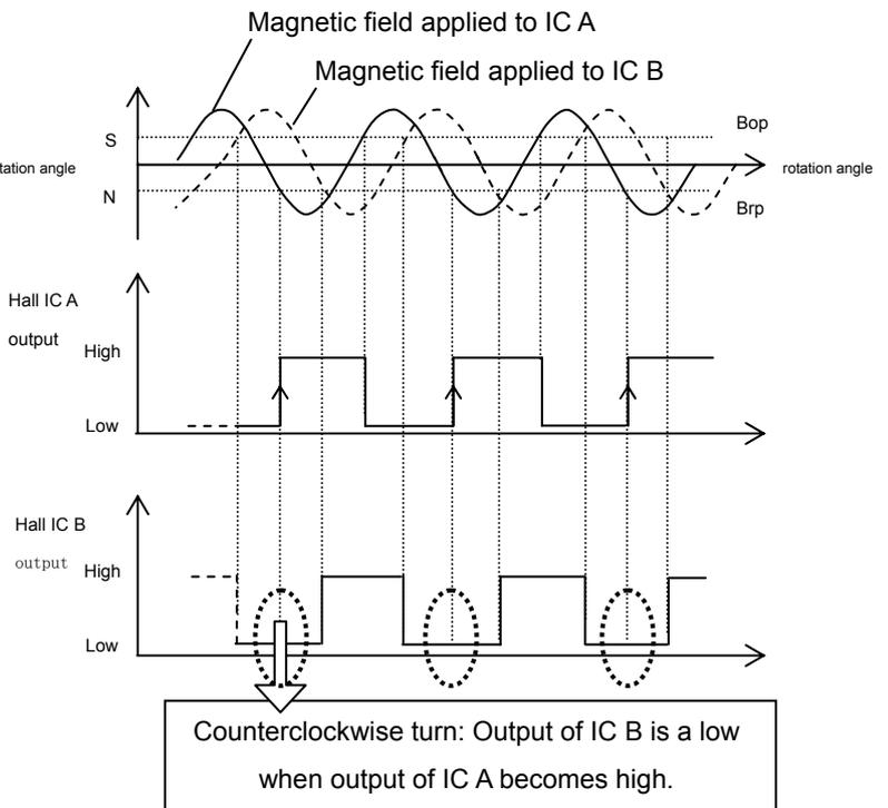
Because the IC measures changes in magnetic field every 1200  $\mu$ S, the IC cannot detect changes in rotation at speeds exceeding this period.
