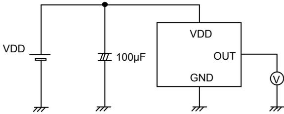
Bop and Brp are measured with applying the magnetic field from the outside.
