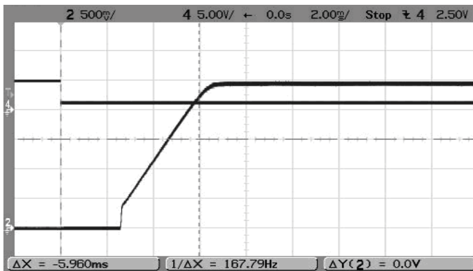
Step Load Transient Response (Vin=12V, Vout=2.5V, Load=0, Iout=1.5A to 3A) Trace 2=Vout, 100 mV/div. Trace 4=Iout, 2.5A/div.
