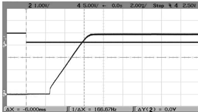
Step Load Transient Response (Vin=12V, Vout=5.0V, Cload=0, Iout=1.5A to 3A) Trace 2=Vout, 100 mV/div. Trace 4=Iout, 2.5A/div.
