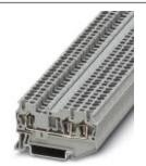
Feed-through terminal block, Connection method: Spring-cage connection, Cross section: 0.08 mm² - 4 mm², AWG: 28 - 12, Width: 5.2 mm, Color: orange, Mounting type: NS 35/7,5, NS 35/15
