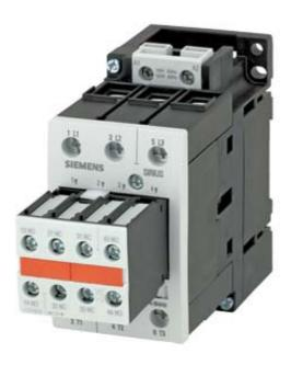
CONTACTOR, AC-3, 15KW/400V, 230V AC, 50HZ, 2NO+2NC, 3-POLE, SIZE S2, SCREW TERMINAL AUX.SW.FRONT BLOCK PERM.JOINTED FOR SUVA APPLICATIONS
