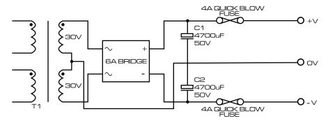
T1 = 100VA 30-0, 30-0 C1/C2 = 4700uF 50V ELECTROLYTICS BRIDGE = 6A 200V PIV
