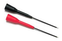
Better than a test probe alone - these two inch long rigid back probe pins easily pass between the weather pack seal and wire. A sharp point ensures good contact to the electrical connector, and the pin's insulation protects it from shorting to other wires.
