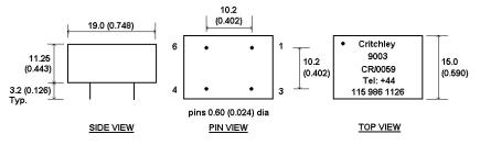
Dimensions in mm (inches) tolerance ± 0.25 (0.01)
