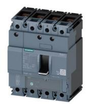
circuit breaker 3VA1 IEC frame 160 breaking capacity class M Icu=55kA @ 415V 4-pole, line protection TM220, ATFM, In=125A overload protection Ir=88A...125A short-circuit protection Ii=10 x In N conductor protection 100% nut keeper kit
