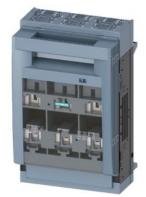
SENTRON, Fuse switch disconnector 3NP1, 3-pole, NH1, 250 A, for Rittal busbar system 60 mm, Box terminal, Cover level 32/70 mm
