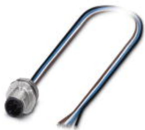
Flush-type connector, Universal, 4-position, Plug, straight, M12-SPEEDCON, A-coded, Front mounting, M16 x 1.5, Individual wires, cable length: 0.5 m
