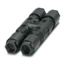
QUICKON H-distributor, black, 4 pos. +PE, 1.0  $\rm mm^2$  ... 2.5  $\rm mm^2$  / 690 V / 20 A, for cable diameters of 9 mm ... 16 mm, with a sealing bolt.
