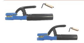
Crocodile electrode holders have a ribbed handle providing a firm grip and good balance. The spring is shielded to prevent damage from spatter and cable fixing is by means of a bolt and copper ferrule (supplied). One of the most popular electrode holders on the market, these are heavy duty.
