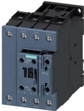
contactor AC-1, 60 A, 400 V / 40 °C, 4-pole, 175-280 V AC/DC, 50/60 Hz, with integrated varistor, auxiliary contacts: 1 NO + 1 NC, screw terminal, size: S2
