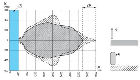
(X): Target distance (Y): Detection limit
