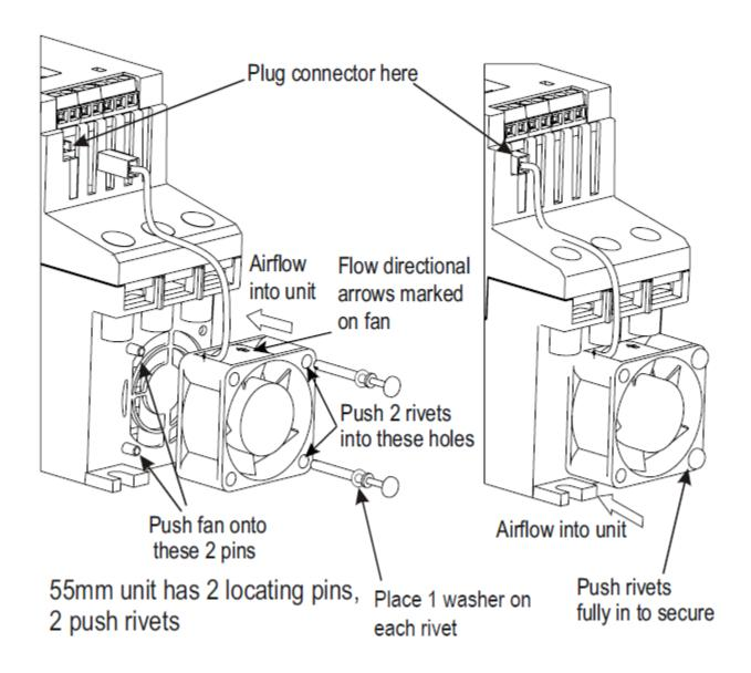
NOTE The RS PRO VMX-PFE soft-starter will automatically detect the fan connection(s), and will adjust its operation accordingly.
