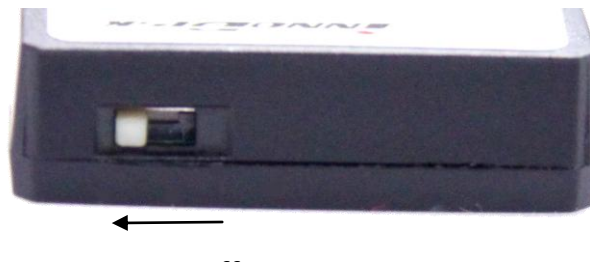
Figure 4: Write Protection Switch Direction
