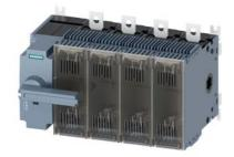
Switch disconnector with fuse 250 A, Size 3, 4-pole for LV HRC fuse Sz. 0 and 1 Front operating mechanism left Complete unit with direct operating mechanism gray flat terminal
