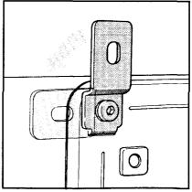
Wall mounting brackets are easily fixed in the vertical or horizontal position.
