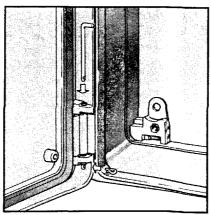
The door may be removed by taking out the locking clip and hinge pin.
