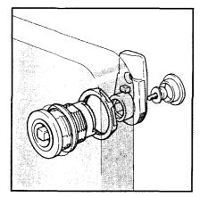
Locks are interchangeable by removing the sealing cap and the Allen screw.
