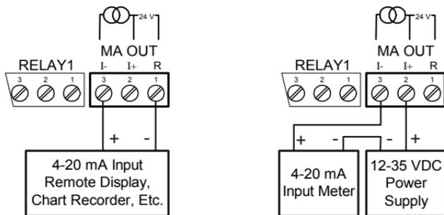
Figure 16. 4-20 mA Output Connections
