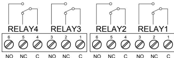
**Figure 12. Relay Connections**
