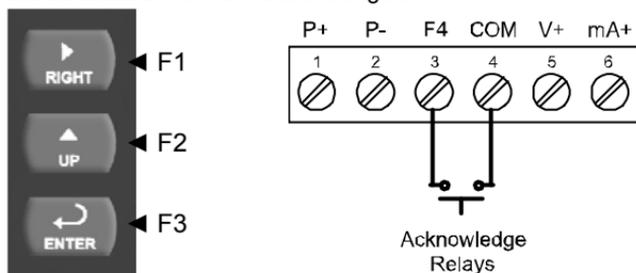
Figure 19. Acknowledge Relays w/Function Key or Digital Input
