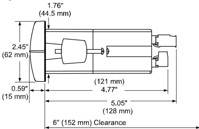
Figure 3. Meter Dimensions - Side View
