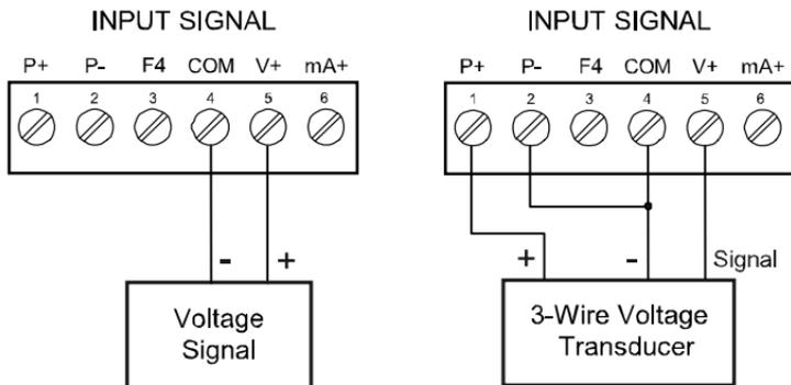
**Figure 11. Voltage Input Connections**
