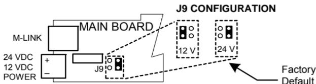
**Figure 5. Jumper Configuration for 12/24 VDC Power
