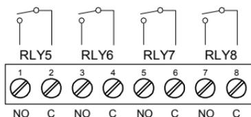
**Figure 17. External Relays Module Connections**
