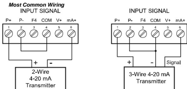
**Figure 9. Transmitters Powered by Internal Supply**
