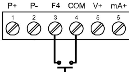
Figure 15. F4 Digital Input Connections
