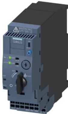
SIRIUS Compact load feeder DOL starter 690 V 110...240 V AC/DC 50...60 Hz 0.32...1.25 A IP20 Connection main circuit: plug-in, without terminals Connection auxiliary circuit: Spring-type terminal
