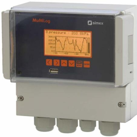
The **MultiLog SRD-N16** device is designed to record and display current values as well as to present technological parameters in the form of charts. The instrument can be equipped with up to eight temperature (RTD / TC), current or voltage inputs, one digital input for the recording process control and one USB Host port for flash data storage. However, due to a significant number of configured parameters it is advised to use the attached configuration software for PCs.
