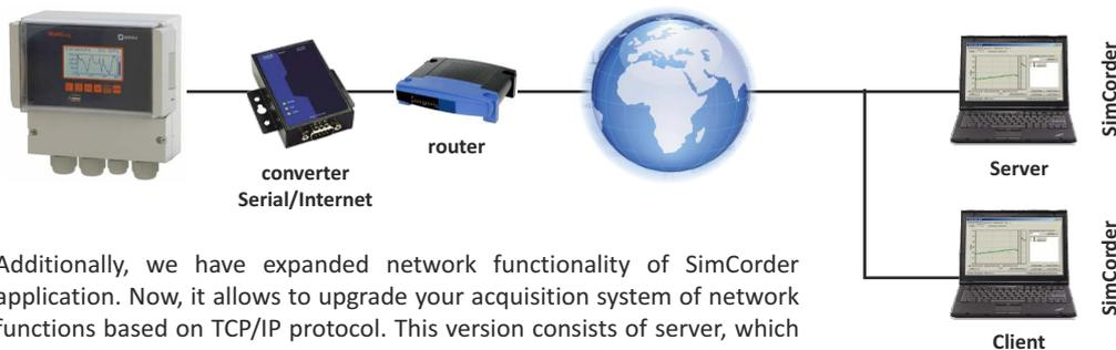
Additionally, we have expanded network functionality of SimCorder application. Now, it allows to upgrade your acquisition system of network functions based on TCP/IP protocol. This version consists of server, which collects measurement data from network and records them to database and clients which communicate to the server and allow watching stored data.
