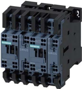
reversing contactor assembly, AC-3e/AC-3, 17 A, 7.5 kW / 400 V, 3-pole, 24 V DC, with integrated diode, spring-loaded terminal, electrical and mechanical interlock, auxiliary contacts: 2 x 1 NO
