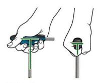
With T-shaped cross-section: broad at the top and slender below. In this way one's hand takes on a firm grip leading to vigorous working over an extended period without any fatigue.
