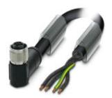
Power cable, 4-position, PUR halogen-free, black-gray RAL 7021, free cable end, on Socket angled M12 SPEEDCON, S-coded, Cable length: 2 m, For AC current up to 12 A/630 V
