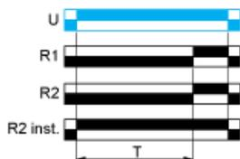
Function Aw : Power On-Delay With Retrigger / Restart Control
