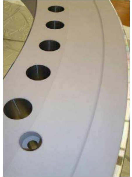
Ring area with SKF High Friction Coating
