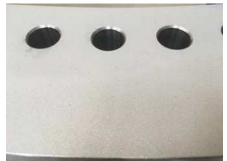
Zinc flame spray coated SKF bearing for a wind turbine
