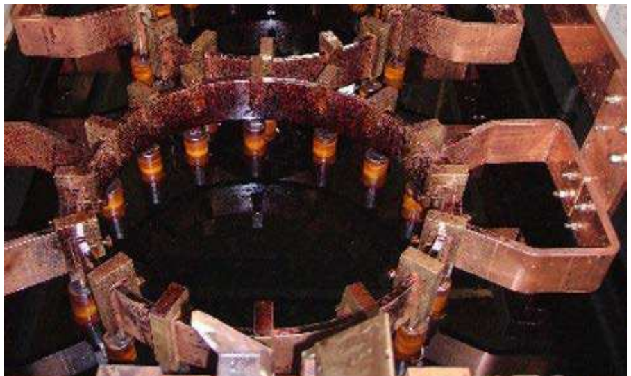
Sophisticated hard chromium anode frames at SKF
