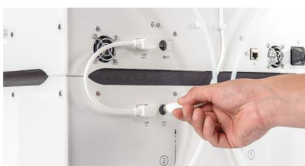
7. Connect the Air Manager cable to the **UMB OUT** port on the Material Station.
