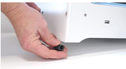
1. Carefully tilt the printer and place the anti-slip feet around the bottom of the frame panels.
