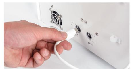
3. At the back of the printer, connect the Air Manager cable to the **UMB OUT** port.
