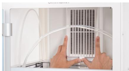
2. Open the door, align the Air Manager filter with the housing, and gently push it into place.
