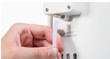
4. Insert the tube coupling collets and Material Station Bowden tubes into the UltiMaker S8 feeders.
