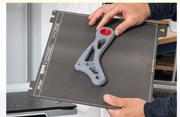
If the object does not detach by bending the plate, you can use a spatula or scraper. Carefully insert the spatula or scraper under the print, parallel to the build plate, and apply some force to remove the print.
