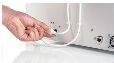
5. Connect the spool holder cable to the NFC socket and secure it behind the cable clips.
