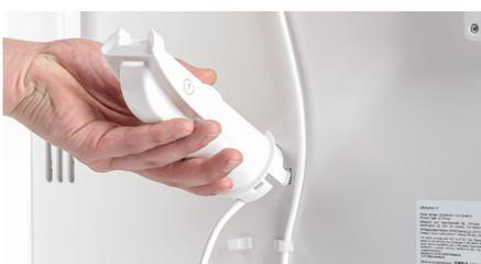
4. Insert the spool holder into the back panel and push until it snaps into place.
