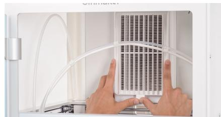
3. Open the door, align the Air Manager filter with the housing, and gently push it into place.
