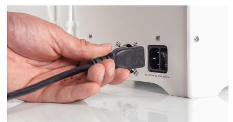
6. Connect the power cable to the printer and the other end to a power outlet.
