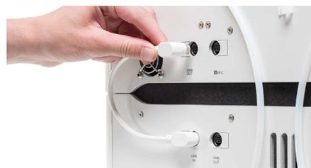
6. Connect the short Material Station cable from **UMB IN** on the Material Station to **UMB OUT** on the printer.
