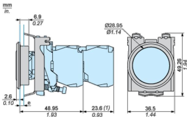
e : Clamping thickness : 1.2 to 2.8 mm / 0.05 to 0.11 in.
