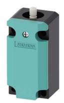
Position switch Basic switch Metal, 40 mm, according to EN 50041 Increased corrosion protection Device connection 1 x (M20 x 1.5) 1 NO/2 NC slow-action contacts functional at -40 °C Shock and vibration test according to EN 61373, Category 1B
