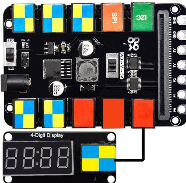
It is compatible with the Micro:bit board and the TS2179 Micro:bit expansion board.
