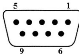
**9 PIN D-SUB FEMALE to LCR Meter (D-SUB2)**
