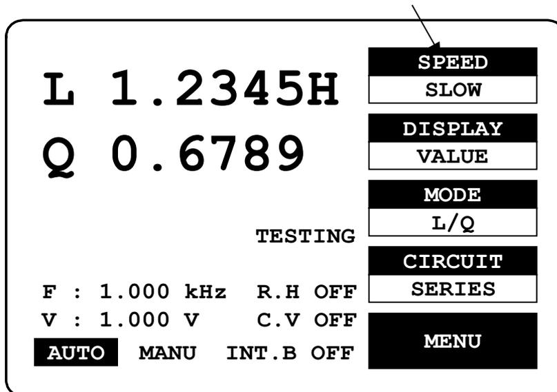
Figure 4-7. Selection of measurement speeds
