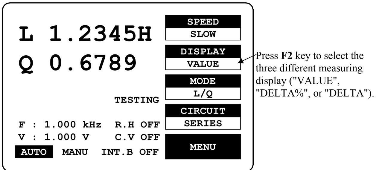
Figure 4-5. Types of measurement display
