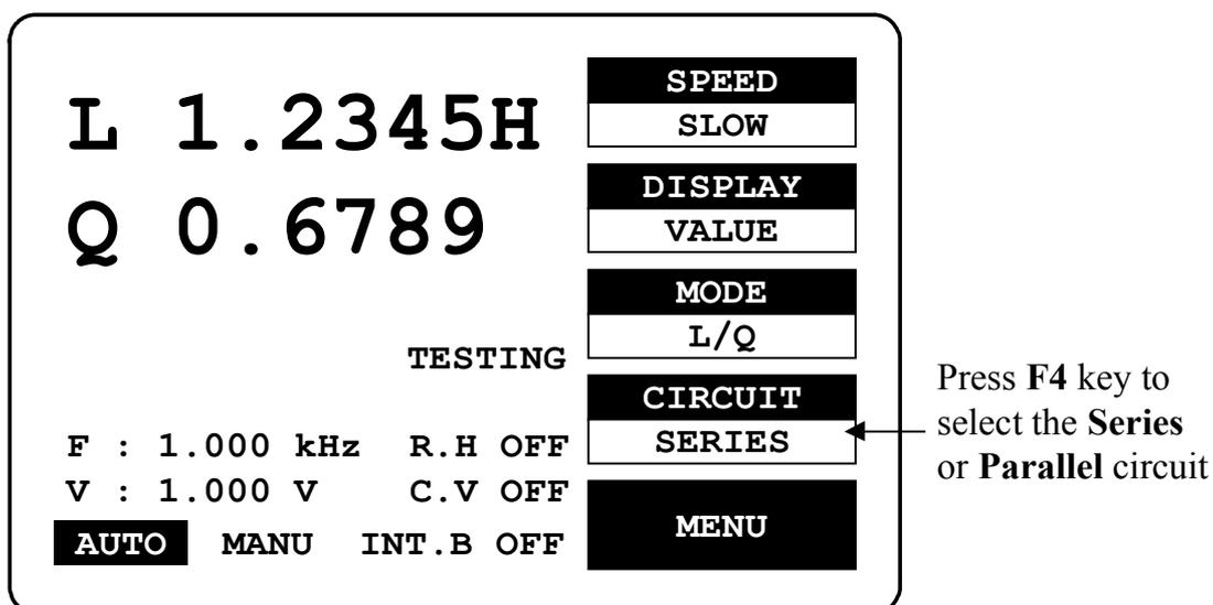
Figure 4-4. Selections of Series & Parallel Circuit
