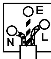
As the colours of the wires in main leads may not correspond with the colours marking identified in your plug/appliance, proceed as follows:
