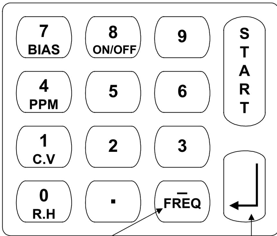
Press - key to input test frequency
