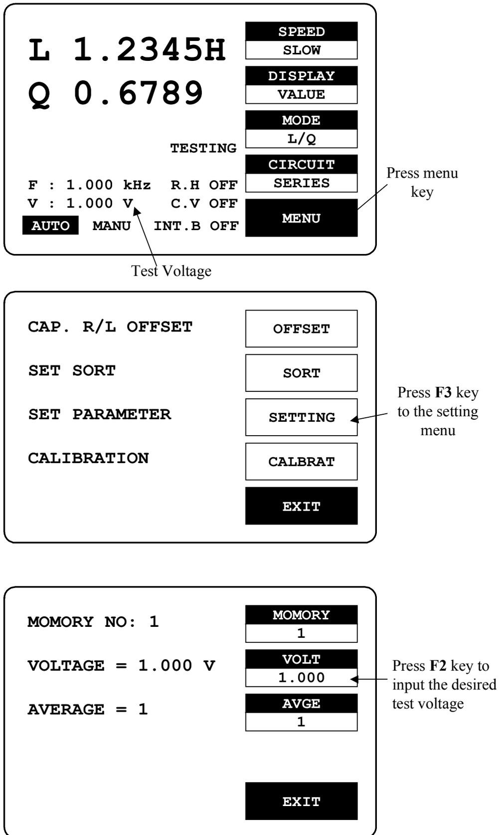
Figure 4-10. Programming of test voltage.
