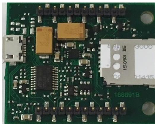
2. Orient the cellular modem as shown and verify the pins are properly aligned.
