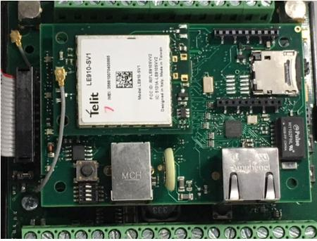
Cellular modem and antenna installed; note that the antenna cable uses the top antenna connection. The LTE modem is shown; the HE910 GSM installation is the same.
