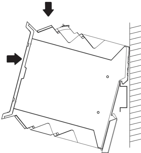
2. Press down firmly to install the interface on a DIN rail.
