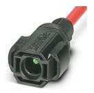
Device connector front mounting, Range of articles: SUNCLIX, color: black, number of positions: 1, min. conductor cross section: 6 mm², Connection method: Crimp, Contact connection type: Pin, cable length: 350
